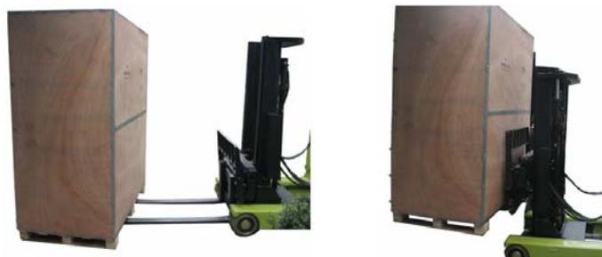
Figure 2-1 Inserting and movement
