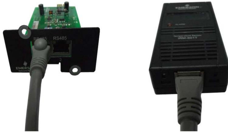
Figure 8-12 Connection between UF-RS485 card and battery temperature sensor
