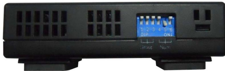
Figure 8-13 Temperature sensor DIP switch
